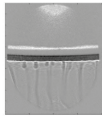
CO 2 dissolution in water at p = 2 Mpa observed by Shadowgraphy from the side 2D configuration
